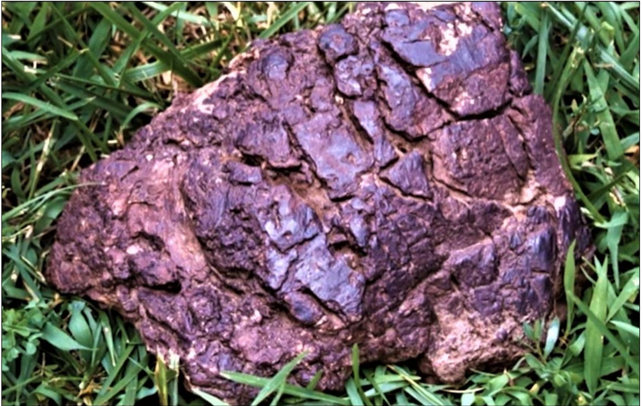
Figure 25: 10-inch-long specimen of ballast material found near the stern (contains 84.14% manganese dioxide, 3.24% aluminum and 0.12% titanium)
